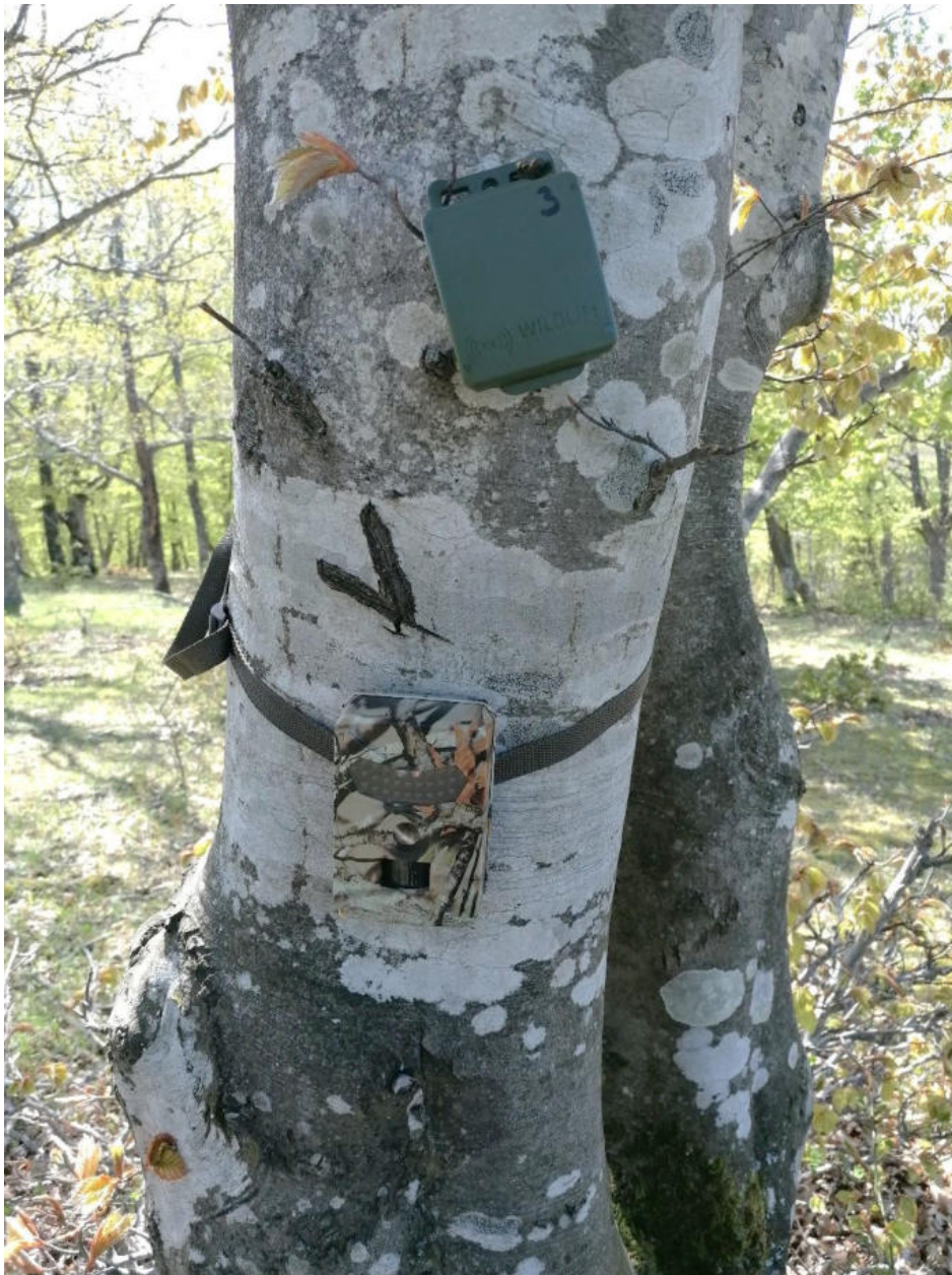
Use of a bio-acoustic station for recording nocturnal predators (top) and a mammal monitoring camera (bottom)
